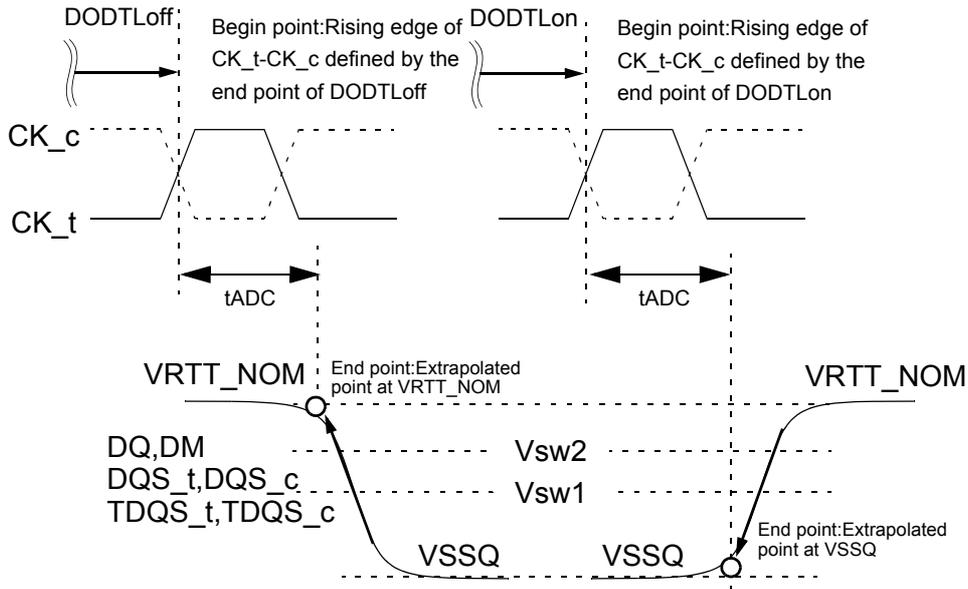
Figure 182. Definition of tADC at Direct ODT Control
