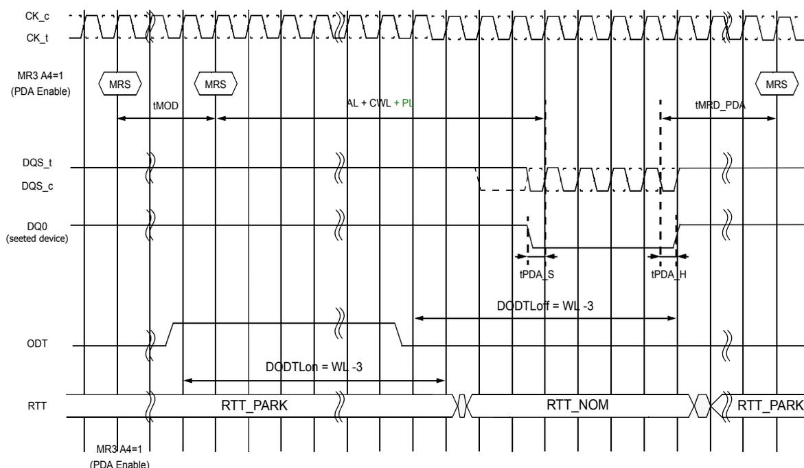
NOTE : RTT\_PARK = Enable, RTT\_NOM = Enable, Write Preamble Set = 2tCK and DLL = ON, CA parity is used
