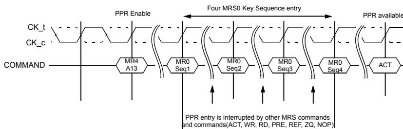
Figure 165. Timing Diagram for soft PPR Key Sequence
