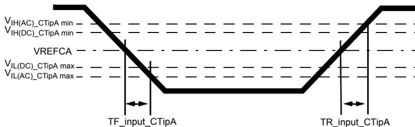
Figure 160. CS\_n and Input A Slew Rate Definition
