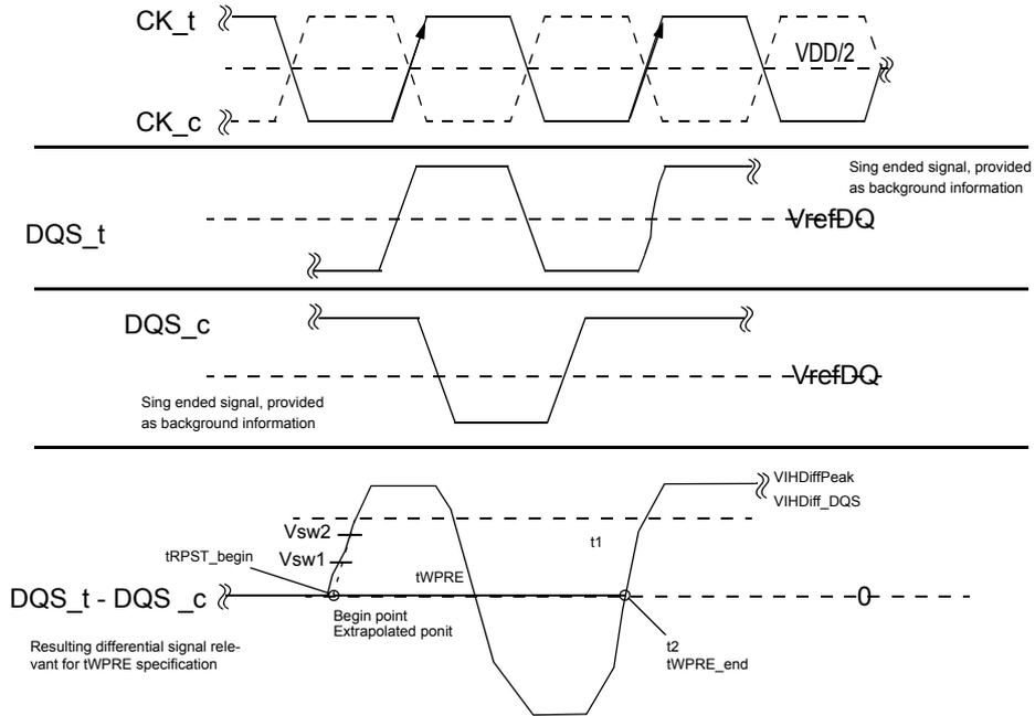
Figure 106. Method for calculating tWPRE transitions and endpoints
