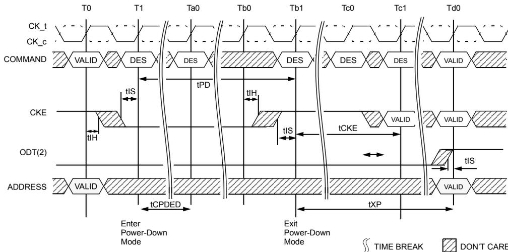
**NOTE :** 1. VALID command at T0 is ACT, DES or Precharge with still one bank remaining open after completion of the precharge command.
