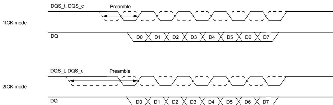
The timing diagrams contained in Figure 60, Figure 61 and Figure 62 illustrate 1 and 2 tCK preamble scenarios for consecutive write commands with tCCD timing of 4, 5 and 6 nCK, respectively. Setting tCCD to 5nCK is not allowed in 2 tCK preamble mode
