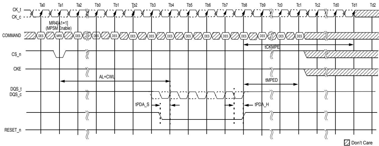
Figure 155. Maximum Power Saving mode Entry with PDA
