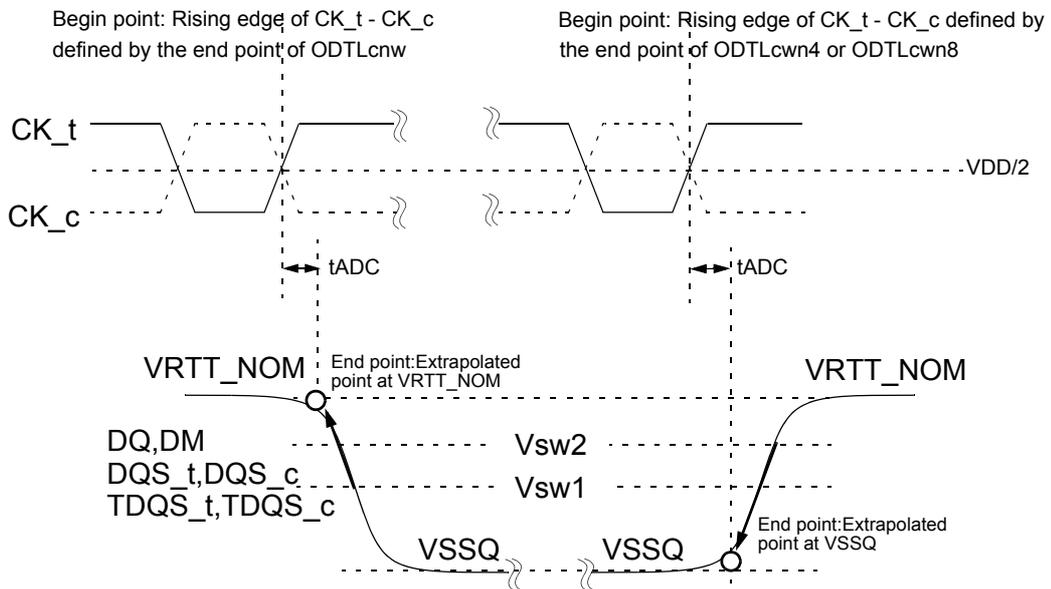
Figure 183. Definition of tADC at Dynamic ODT Control
