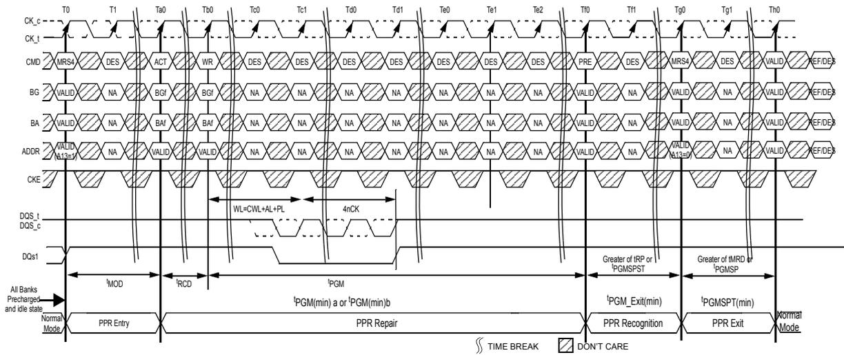
**Figure 167. Fail Row Repair (WR Case)**
