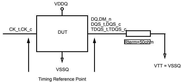
Figure 181. ODT Timing Reference Load
