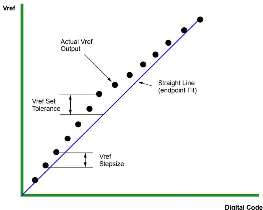
**Figure 22. Example of Vref set tolerance(max case only shown) and stepsize**
