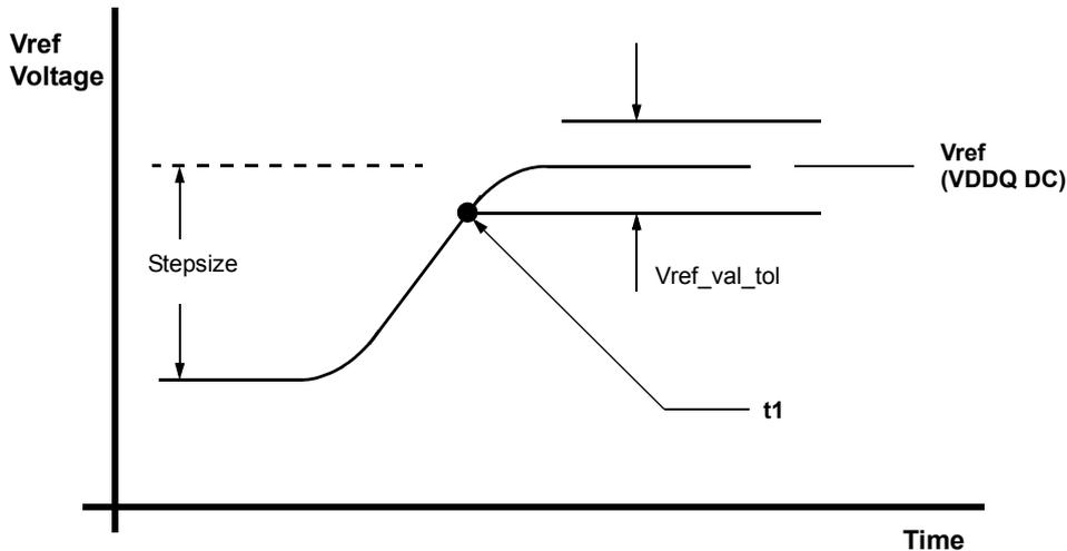
Figure 25. Vref step single stepsize increment case
