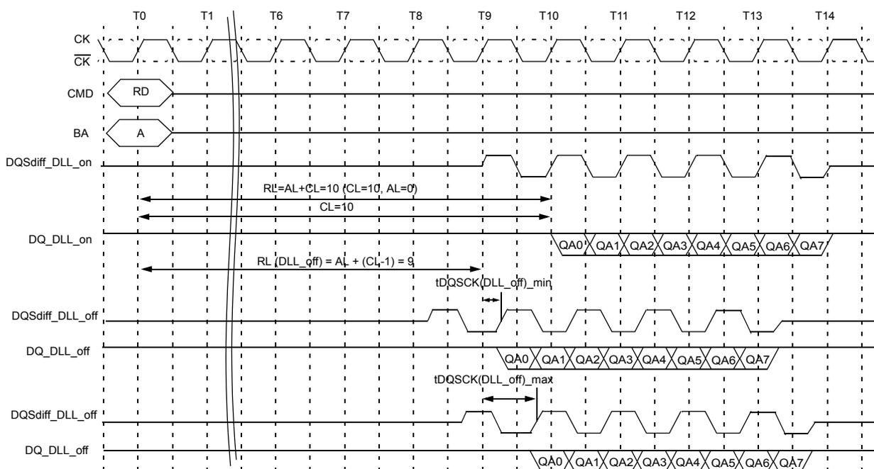
Figure 7. READ operation at DLL-off mode
