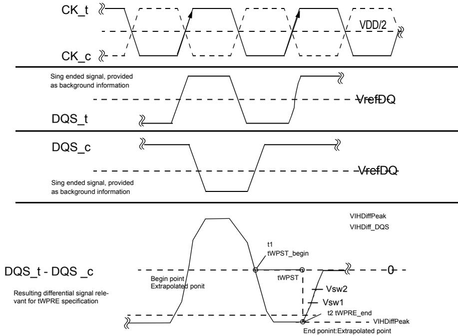
Figure 107. Method for calculating tWPST transitions and endpoints
