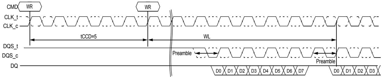
2tCK mode:  $t_{CCD}=5$  is not allowed in 2tCK mode
