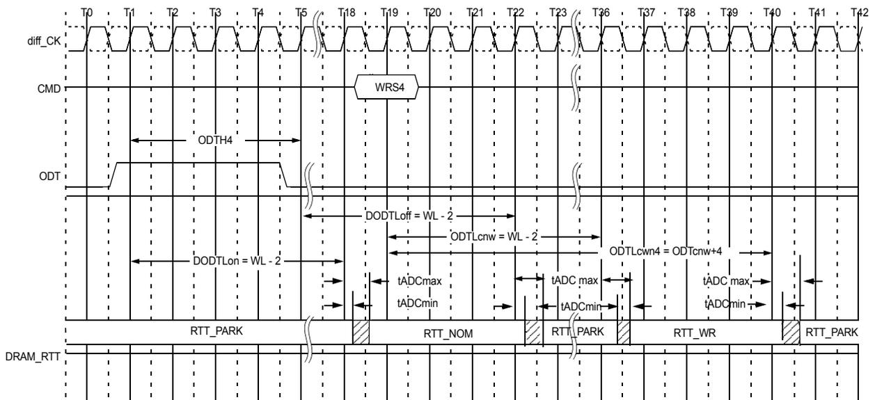
**Figure 174. Synchronous ODT example with BL=4, CWL=9, AL=10, PL=0; DODTLon/off=WL-2=17, ODTcnw=WL-2=17**
