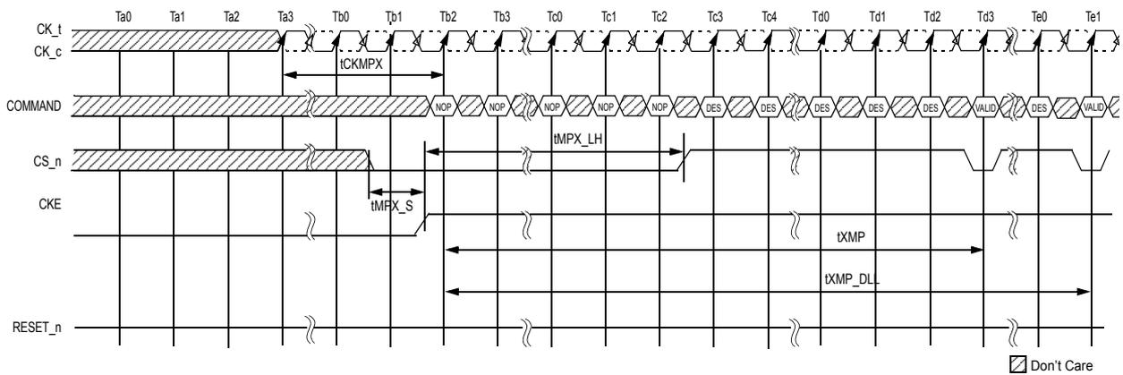
Figure 157. Maximum Power Saving Mode Exit Sequence
