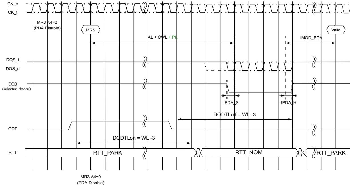
NOTE : RTT\_PARK = Enable, RTT\_NOM = Enable, Write Preamble Set = 2tCK and DLL = ON, CA parity is used
