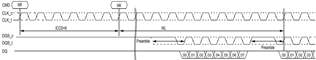
Figure 62.  $t_{CCD}=6$  (AL=PL=0)
