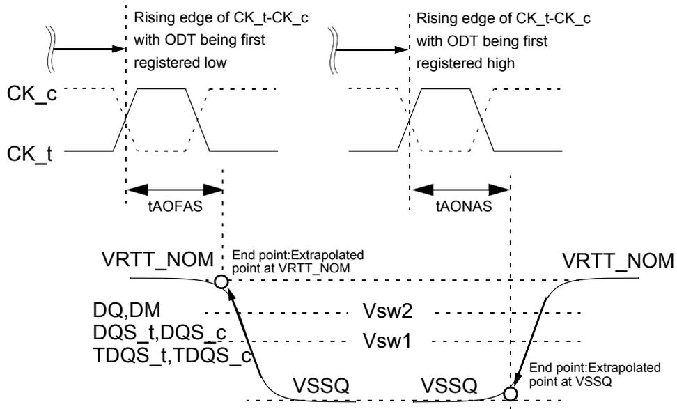
Figure 184. Definition of  $t_{AOFAS}$  and  $t_{AONAS}$
