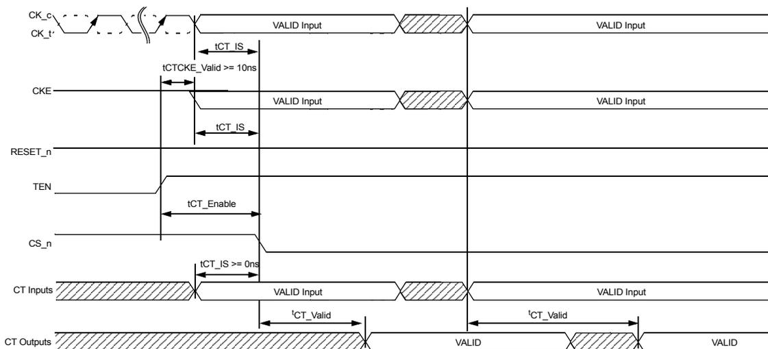
Figure 158. Timing Diagram for Connectivity Test(CT) Mode
