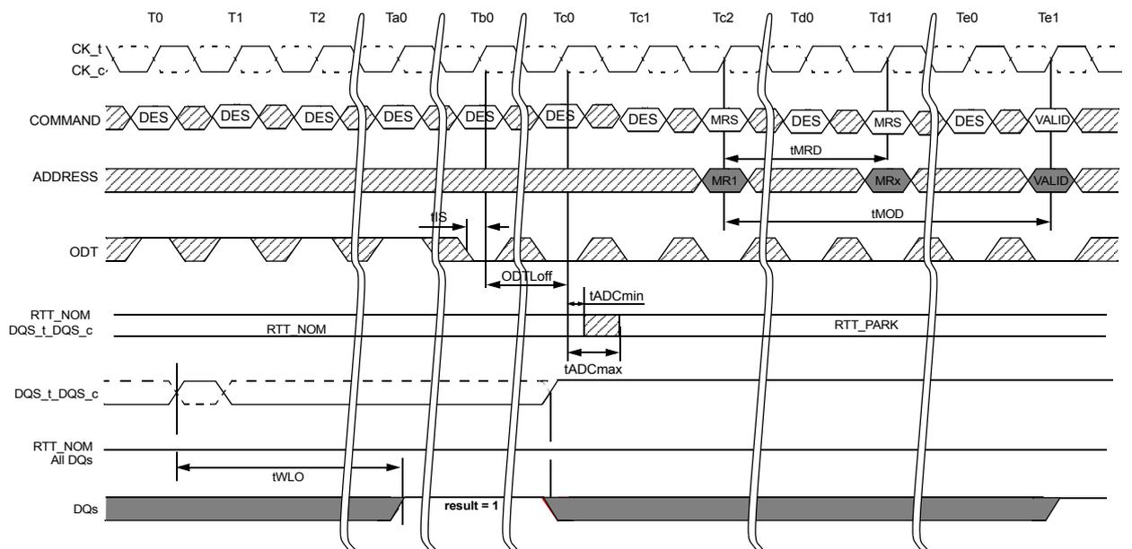
Figure 10. Timing details of Write leveling exit
